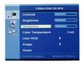
b. Press " $\triangle$ " or " $\nabla$ " to increase or decrease the sharpness of the display. Press "1" to confirm the adjustment and back to OSD main menu.
